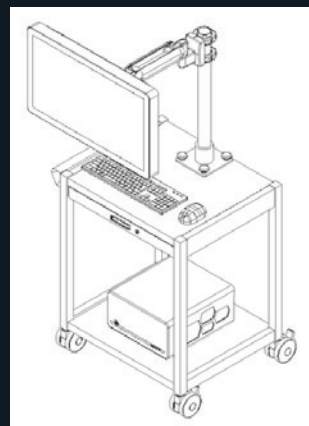
MOBILE WAGON W x D x H: 660 x 550 x 1434.5 mm (excluding monitor)
